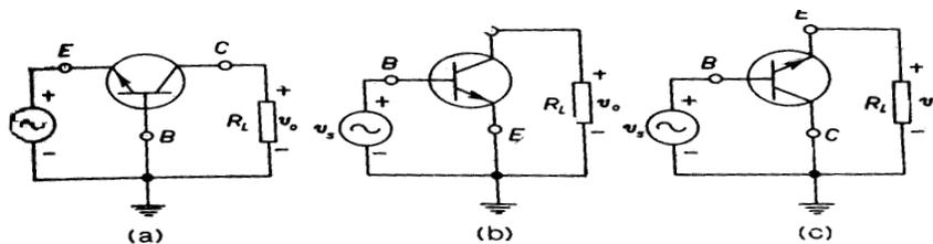
Fig 6.19 Configuration of transistor (N P N Type)
