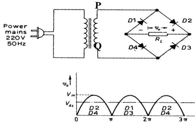
Fig 7.4 Bridge Rectifier
