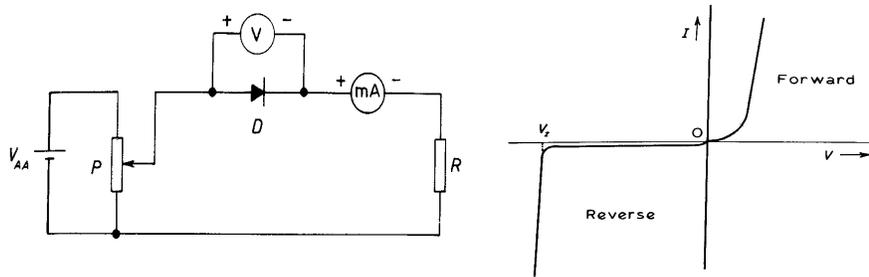
Fig 6.11. V I characteristics of PN junction diode.
