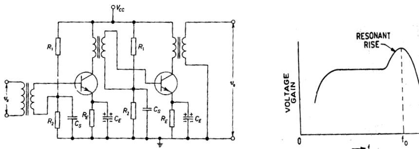
Fig 8.11 (a) Transformer coupled amplifier
