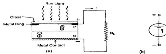
**Fig 6.17 Solar cell (a) Basic consists (b) Symbol**
