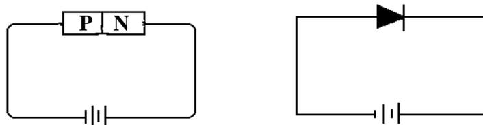
Fig 6.10 P N junction with Reverse bias.
