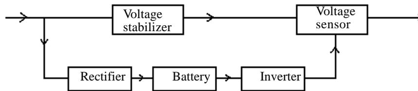
Fig. 7.14 Block diagram of UPS
