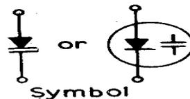
**Applications:** It is used in T.V. receivers, Radio receivers, Communication equipments.
