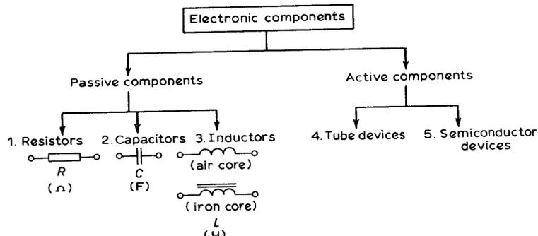
Fig 6.1 Types of Electronic components.
