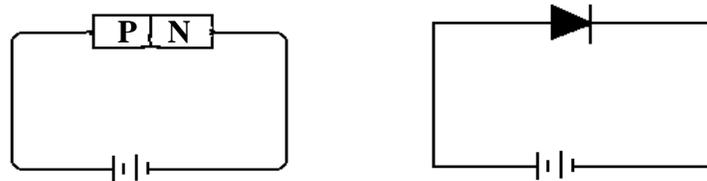
Fig 6.9 P N Junction with forward bias
