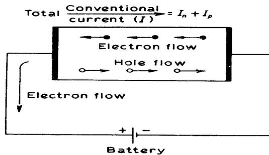
Fig 6.5. Conduction of Current in an intrinsic semiconductor
