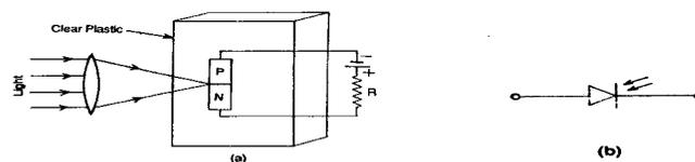
**Fig 6.18 Photo diode (a) Basic Construction (b) Symbol**
