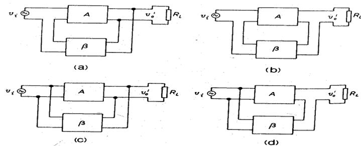
(a) Series-voltage feedback; (b) Series-current feedback;
