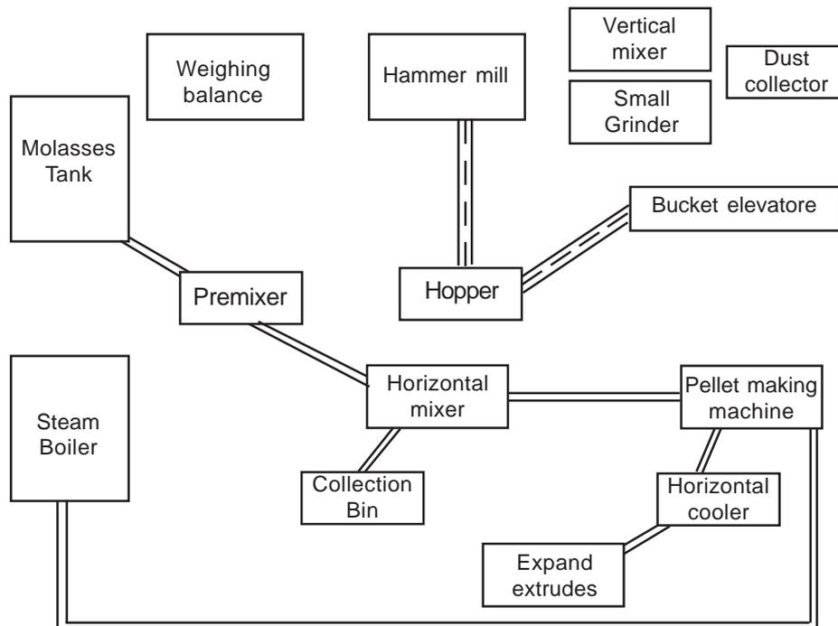
The layout or arrangement of different equipment and work area is important for efficient plant operation. The arrangement, either installed or in plan includes the space needed for material movement, storage, indirect labourers and all other supporting activities or services, as well as for operating equipment and personnel.
