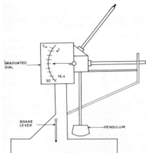
**2. CHARPY TEST:** The specimen to be tested is 10mmx10mm in cross-section and 60mm long having a standard 45° notch 2mm deep in the center. The specimen is mounted horizontally between the two anvils with a clear span of 40mm. The specimen shall be placed such that the notch is on the other side to that of striking edge.
