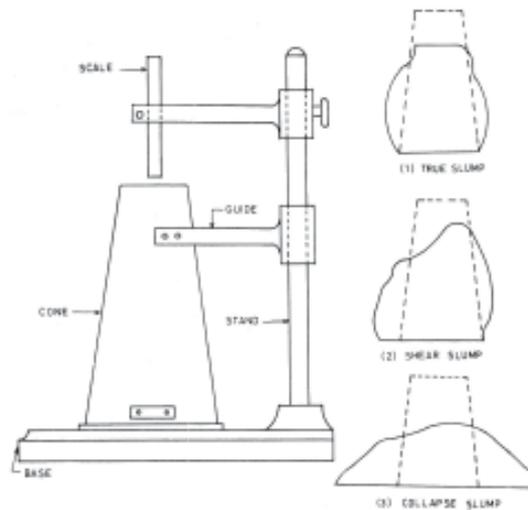
Fig. 6.2 The Slump Cone kinds of Slump
