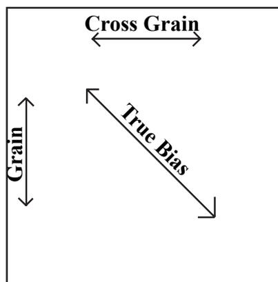
Fig: 15 Indication of Grain on the Fabric
