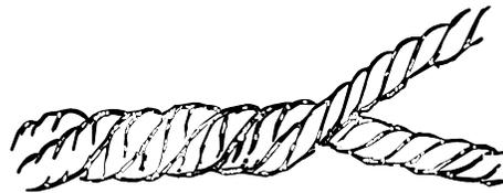
**Fig :13 Twist on twist 2 - Ply Yarn**
