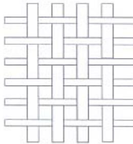
**Twill Weave:** A twill weave is characterized by diagonal lines on the face or the back of the fabric. For example denim. This weave requires a minimum of three harnesses for manufacturing. High strength and compact weaving characterize twill weave. These fabrics have good abrasion resistance and are durable. The direction of the twill can be varied to create interesting effects such as right hand twill weave, left hand twill weave, broken twill weave, pointed twill, herringbone etc.,
