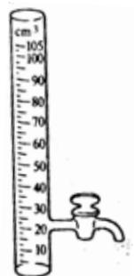
They are pair of cylinders employed in matching colours by balancing method. Each cylinder has a glass stop cock about 2.5 cm. from the bottom. Through the stop cocks liquid can be withdrawn until colours in the two cylinders match on observing vertically. They are graduated in ml.s and have capacity of approximately 100 ml.
