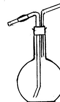
Wash bottle is a flat bottom flask, that delivers distilled water or other liquid for use in the transfer and washing of precipitates. It is fitted with a rubber bung with three holes. By mouth, air can be pumped in to force the liquid through the other tube. Third tube will be open at both ends and should be closed by thumb while water is being blown out. It should be removed when the mouth pressure is released. It is used when organic
